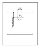
Non-threaded Hex shaft with PR-D-30H-PU-N
