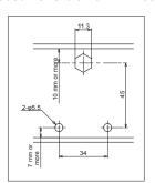
Non-threaded Hex shaft with PR-D-30H-PU-N-ST
