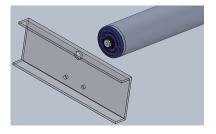
NOTE: Collar part is 4 mm out for  $\phi48$ and φ50 Motor Roller.
